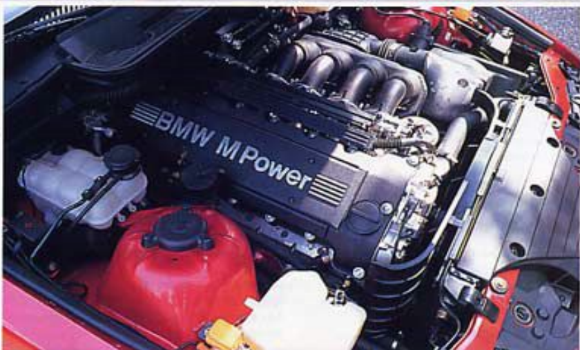
M3's 3-litre twin-cam straight-six boasts 286bhp and 236lb ft of torque
